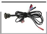
Emulation/acquisition cable, with PWM power generator function such as PWM POWER with integrated 5V voltage generator; mass generator and control of the Feedback. It is used for the activation of feedback controlled components via potentiometers
